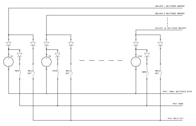
It is strongly recommended that each motor is fitted with a 100nF capacitor and back emf protection diode (cathode to +ve side of the motor) directly across the motor terminals.
